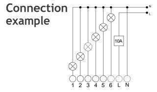
This module is designed For smooth adjustment oF brightness oF lighting devices (non reactive load). The dimmer type is MOSFET with trailing edge dimming.
